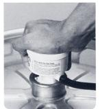
3. Rotate the pump body one-quarter turn clockwise to engage the keg lugs. (This locks the pump in place and opens keg valve).
