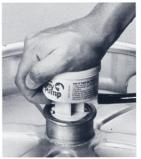
**2.** While holding firmly in a vertical position, press pump body down onto the keg valve.
